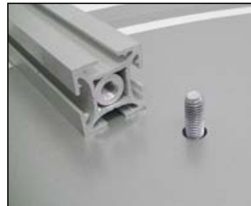
Base Plate Connection
